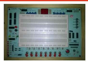
Excel's Digital Trainers have been designed with the idea of providing basic facilities essential for conducting simple experiment in the Laboratory. Using these facilities one can get familiarized with the various Digital ICs.
